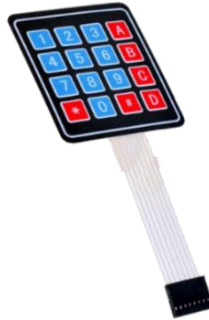
Gambar 2. 10 Keypad Matriks 4x4
