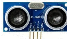
Gambar 2. 2 Sensor Ultrasonik HC-SR04
