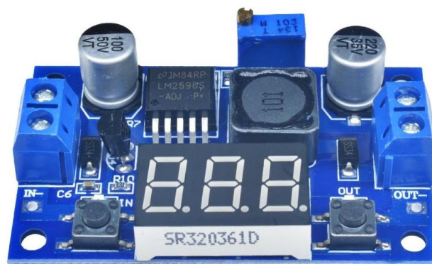
Gambar 2.4 Regulator Tegangan ( Buck converter )
