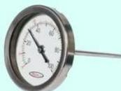
Gambar 3 Termometer Bimetal
