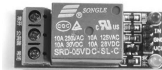
Gambar 2. 3 Modul *Relay* Arduino
