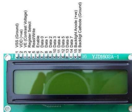
Gambar 2.3 LCD (*Liquid Crystal Display*)
