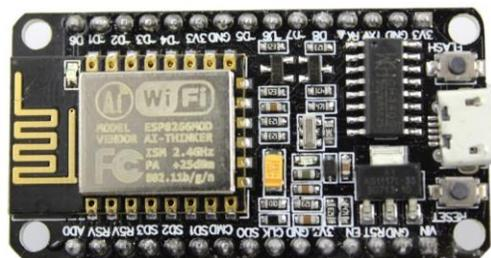
Gambar 2.2 NodeMCU ESP8266
